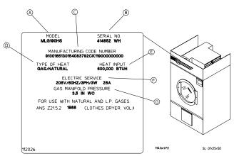
When contacting ADC, certain information is required to ensure proper service/parts information. This information is on the data label, located on the top right corner of the dryer, viewed from the rear (refer to illustration). When contacting ADC, please have the model number and serial number readily accessible.
